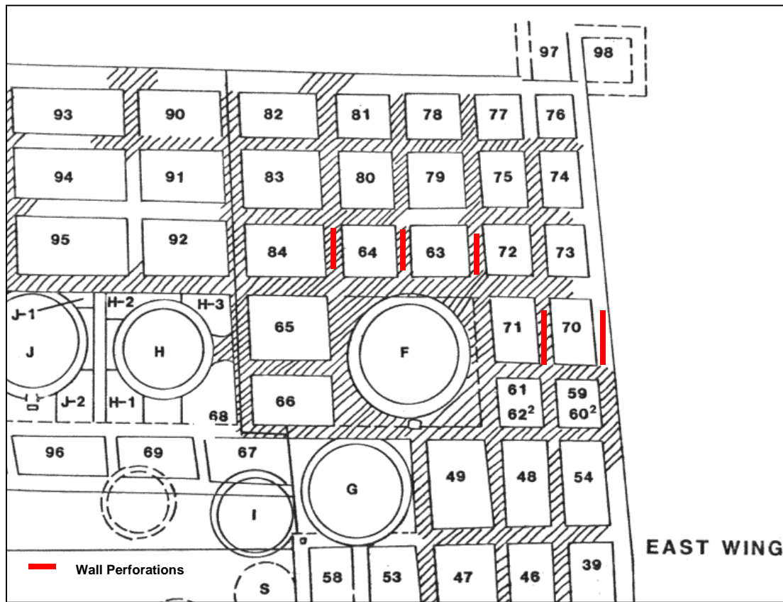
Figure A1. Location of wall perforations in FY00 backfill area.
